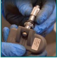
Once the original sensor is removed, clear the stem hole of any dirt. Program new sensor (if applicable, see STEP 2) Then insert the new valve and sensor into the stem hole, followed by the washer and nut. Tighten the nut to 4Nm.
