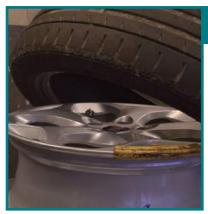
Place the wheel on the turntable and demount the tyre. The sensor can then be removed.
