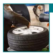
Reinstall the tyre, making sure no contact is made with the new sensor to prevent damage. The tyre, complete with TPMS sensor, is now ready for inflation to the correct PSI level.
